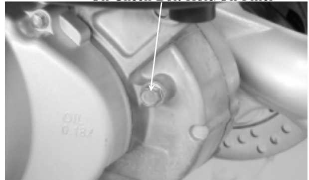
Oil Check Bolt Hole/Oil Filler
